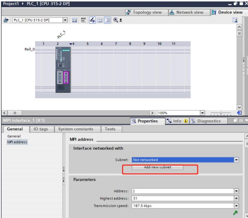
5. It will generate "MPI\_1" network. The "Address" should match the MPI address of PLC. The default is 2.
